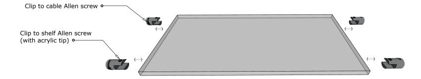
Attach 2 **shelf/cable clips** to each side of each glass shelf. Each glass shelf requires 4 clips. Follow dimensions on next pages to ensure all clips are installed on each glass shelf in the same position so that shelves are in line when attaching them to the cables. Allen screws are provided.
